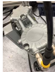
Figure 3-5 Connecting the manifold with GAST pump.
