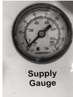
Figure 4-2 Observe the Supply gauge (-85 kPa)
