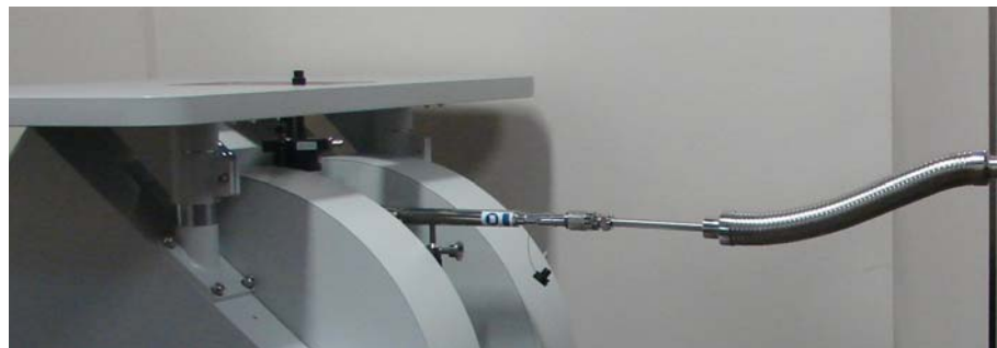
Figure 3-10 Bayonet inserted into cryostat
