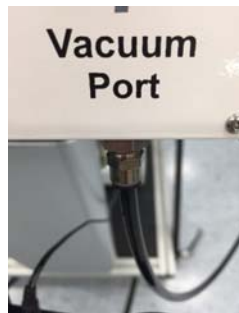
Figure 3-5 Connecting the manifold with GAST pump.
