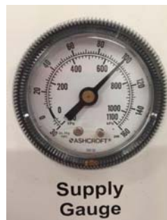
Figure 4-6 Supply Gauge 690 kPa (100 psi).
