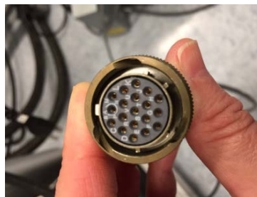
Figure 3-11 19-pin connector on instrumentation cables.
