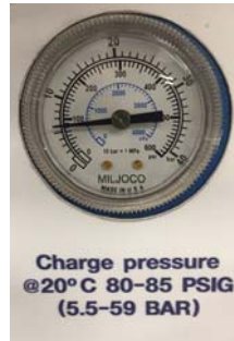
Figure 4-5 Recirculator Charge Pressure.
