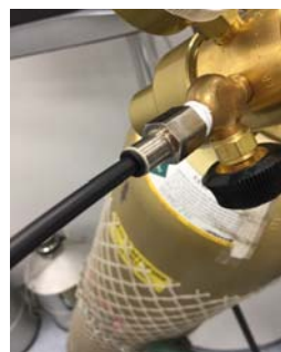
Figure 3-6 Connecting the manifold with helium cylinder.
