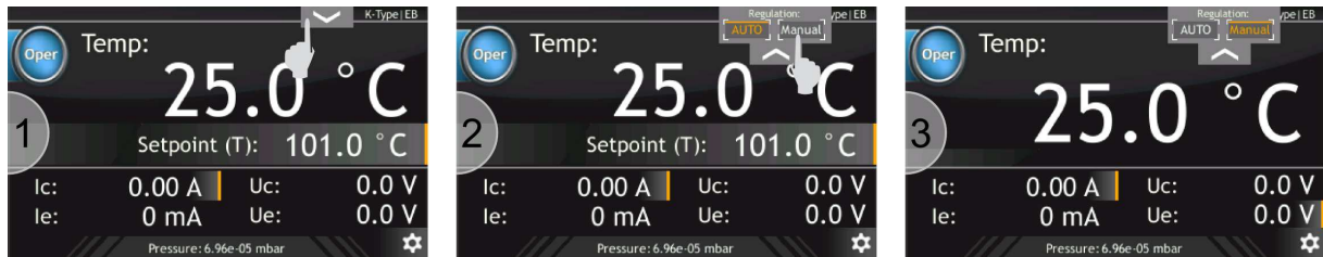
Figure 3.45: Setting manual regulation for electron bombardment
