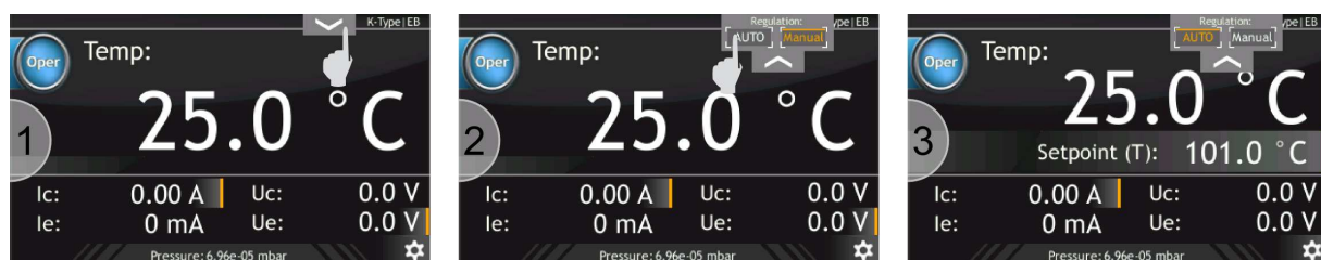
Figure 3.44: Setting AUTO Regulation for electron bombardment
