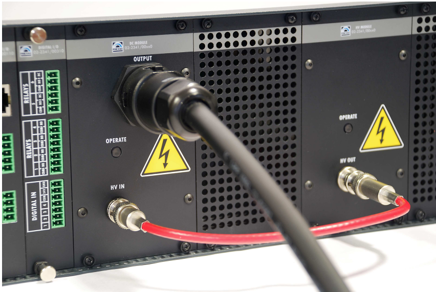
Figure 2.10: Connection necessary for proper operation in Electron Bombardment mode
