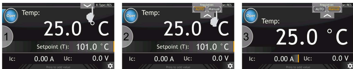
Figure 3.43: Setting manual regulation for resistive heating
