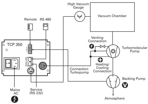
Fig. 3: General overview of the connections on the TCP 350
