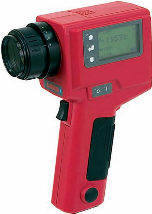
Fig. 1-1 Land Cyclops 160B portable infrared thermometer
