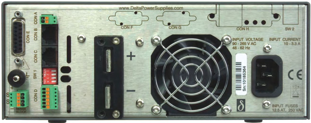
fig. 2 - 8 Location of output terminals and analog programming connector on the rear panel (standard unit)
