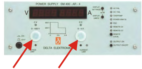
fig. 2 - 23 Screwdriver adjustment at front panel. Behind the plastic caps, the CV- and CC-settings can be adjusted with a screwdriver.
